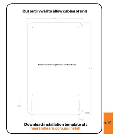
**Installer responsible** for ensuring cabinet is mounted to secure stud or similar **250mm** 368.5mm See following page for detailed wall mounting **Cabelling to exit-location** as we determine hole location
