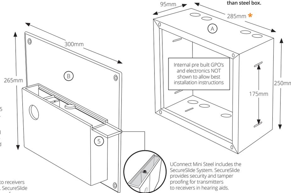
UConnect Mini Steel includes the SecureSlide System. SecureSlide provides security and tamper proofing for transmitters to receivers in hearing aids.
