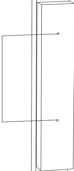
Screw fix UConnect Mini box to in wall carpentry. Spacers may be required.
