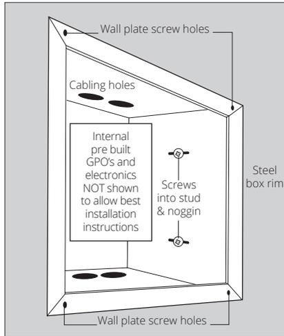
Mount steel box so plaster / wall surface is flush with steel box.
