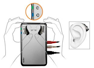
(2) Hold both hearing aids close to the transmitter. The pairing process starts automatically. The LEDs will turn blue for 30 seconds, indicating that they're pairing.
