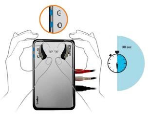
4 A medium press / hold / release of 1-3 seconds on the rocker switch of the hearing aids will initiate TV streaming.
