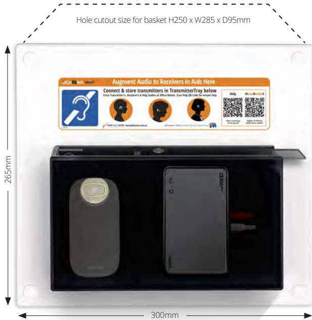
The UConnect Mini Wall Panel is mounted 1000mm from the bottom edge to the floor. It must be unobstructed and in line of sight to all learners in the learning space.
