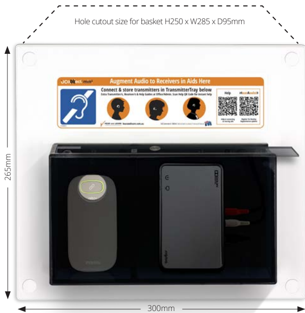
The UConnect Mini Wall Panel is mounted 1000mm from the bottom edge to the floor. It must be unobstructed and in line of sight to all learners in the learning space.
